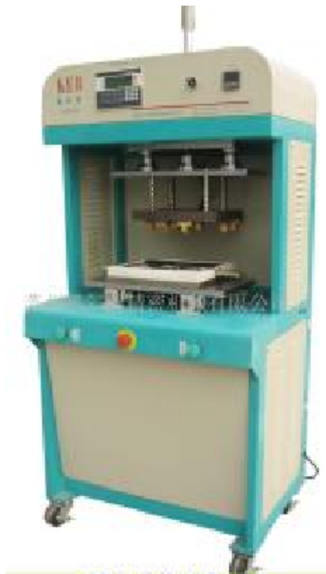
图20 埋植螺母热熔
